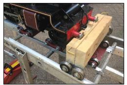
without any manual lifting. As can be seen in the photos with a couple of bits of timber and some roller bearings for wheels I cobbled together a gadget to support the loco as it is moved into position over the rollers. A trolly jack being used to lift the loco about 10mm to get the loco on and off the wood block. The two bits of brass you can see in the picture slide behind the buffers to prevent the loco slipping off the
