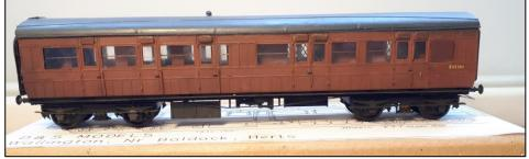
A key feature of the build of these and my restaurant car is fully compensated running gear which works on the "three-point suspension" principle meaning that all wheels are on the rails at all times.
