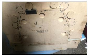
A jig has been made to help form/weld the valance end sections to the specification we gave but has since been altered to allow them to be made longer. The plan is for "longer" one end section to be made which can be attached to one of our existing carriages once the site reopens. It can then be
