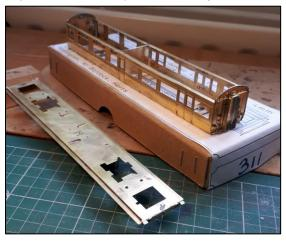
for which I use 3 different solders of various temperatures with fluxes to match. The trick to the soldering is to keep a very clean iron tip (not easy with the aggressive fluxes) and very clean components. It also helps various cunning have to methods to hold components in place when applying heat especially the tiny pieces which have a habit of trying to stick to the tip of the iron rather than stay on the model. Fingers are useless (they burn) but
