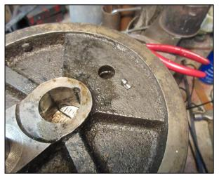
axle in service and would no longer perform as it should because this movement had thrown the timing out. The wheel was made as a push fit on the axle the problem now was how to get the grub screw out; I did not want to risk drilling out what was left of the screw so decided to push the wheel off the axle and repair the resultant damaged thread. Fortunately, the threads on the grub screw gave up without a fight and the Axle
