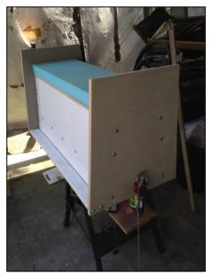
rectangles front and back and fitted it with some old dexion angle, but I did not like the way this was looking, it was too box like. So, I angled the sides 5 degrees. and sanded the ply ready for painting. The result wasn't very good so tried a different approach with some old beechwood cupboard doors which I cut to the thickness of the ply. I then machined a tongue and groove joint, applied adhesive and clamped the lot up. The finished appearance with a coat of acrylic paint was much better.
